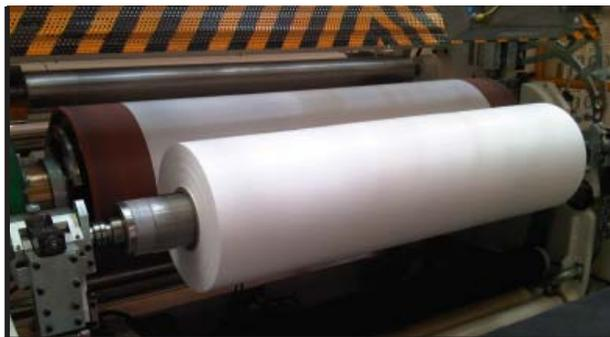
① The three-layer functional PP film is characterized by very high vapor permeability - Sd in the range from 0 to 0.04 [m]. The diffusion of water vapor is associated with micropores, which diameter is several hundred times smaller than the diameter of a drop of water. They are created in the process of extrusion during the production of a PP film with the addition of chalk. The microporous PP film is both watertight and vapor-permeable.
